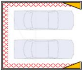
Fig. 1 Standard Double Garage 6m x 6m Standard Single Garage 4m x 6m Area requiring Additional Mechanical Protection (such as a Bollard) Area deemed protected by the garage pillar or wall, not requiring additional protection. As a guide the protected area is calculated at ratio 1 : 2.5 i.e: 500mm garage pillar, would allow an area of 1250mm protection along the wall. Each installation must be assessed for potential hazards and any reduction methods implemented.
